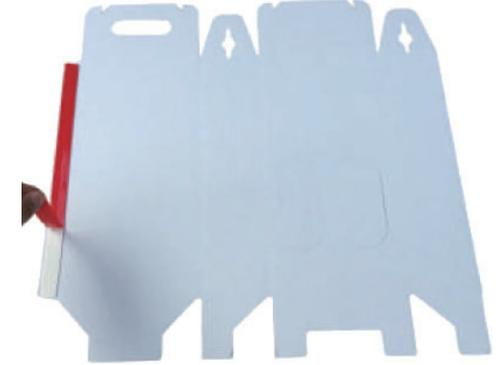
2. Fold up the end flap from the other side, and attach it onto the double sided tape. Be sure the edge align with the crease. Apply pressure to make sure the tape fully contact with the cardboard and the edge is secure.
