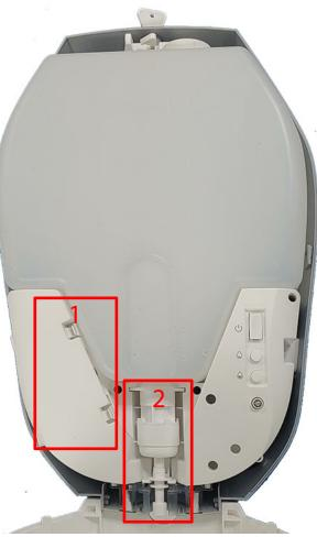
2. Before replacing the liquid container, extend the highlighted bracket to the bottom. The bracket must be sandwiched in between 2 round plates on the dispensing stem.
