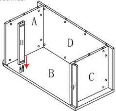
5. Insert (11) cam posts into another Panel B. Install Swing Door G onto assembled panels with sign facing outside, and hold it at its place. Assemble the 2nd Panel B with rest panels by inserting the cam posts into corresponding holes.
