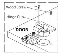
(c) Hold the door with concealed hinge assembled, and align holes in the hinge plate with pre-drilled holes in Panel B. Drive wood screws into pre-drilled holes to fix the door panel.
