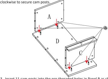
3. Insert 11 cam posts into the pre-threaded holes in Panel B as shown below. Attach the assembled panels in STEP 2 to Panel B and use cam locks to securely lock it in place.
