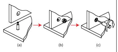
2. Screw 4 cam posts into the holes in Panel D. Attach Panel A and assembled Panel C to Panel D. Insert 4 cam locks into cam lock holes on Panel A and Panel C, use a phillips screw driver to rotate cam locks
