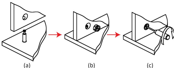
2. Screw 4 cam posts into the holes in Panel D. Attach Panel A and assembled Panel C to Panel D. Insert 4 cam locks into cam lock holes on Panel A and Panel C, use a phillips screw driver to rotate cam locks clockwise to secure cam posts.
