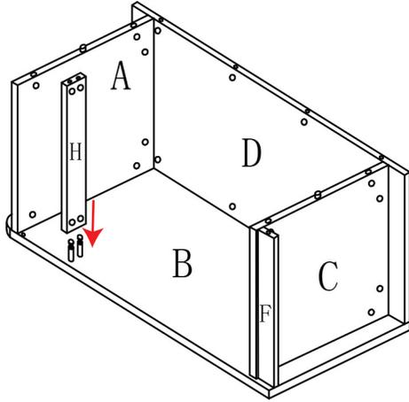
5. Insert 11 cam posts into another Panel B. Install Swing Door g onto assembled panels with sign facing outside, and hold it at its place. Attach the 2nd Panel B to the assembled receptacle body by inserting the cam posts into corresponding holes, then insert and tighten cam locks.
