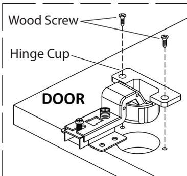
(c) Hold the door with concealed hinge assembled, and align holes in the hinge plate with pre-drilled holes in Panel B. Drive wood screws into pre-drilled holes to fix the door panel.
