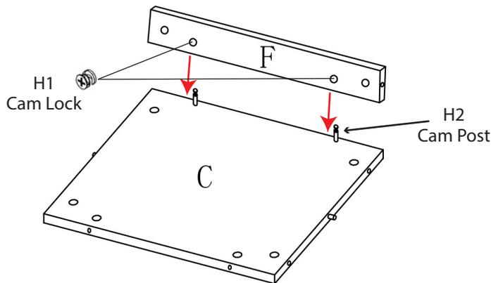
How to join 2 boards with CAM lock:
