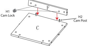
How to join 2 boards with CAM lock:
