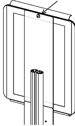
Step 6. Attach the hand sanitizer dispenser to the Bent Acrylic: Align holes visible on the inside of the sanitizer dispenser with corresponding holes on the Bent Acrylic.
