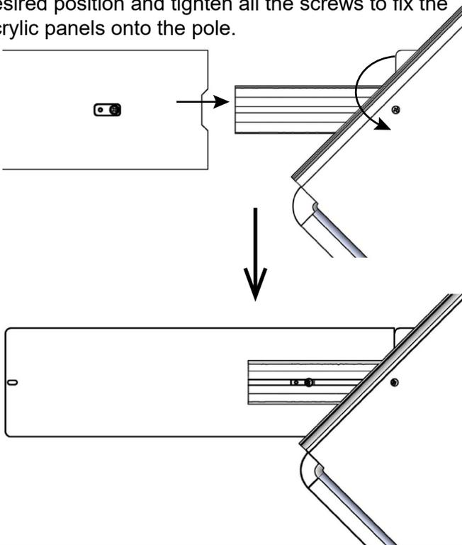
Step 5. Rotate the Snap Frame back to its display position and align the top hole with the top slot on the Acrylic. Screw (1) M4X14mm through the aligned holes from the front and tighten it with (1) Square Nut.
