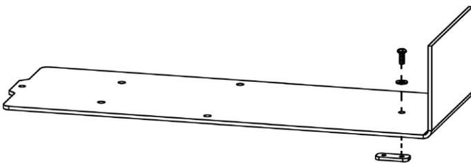
Do not fully tighten the screw and the nut, leave them loose for inserting into T-slot.
