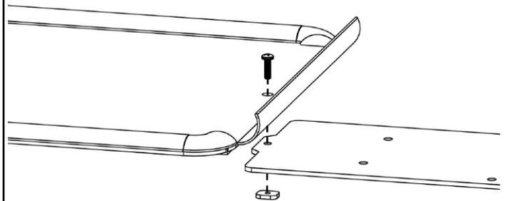
Do not fully tighten the screw and the nut. Leave a gap between nuts and the Bent Acrylic
