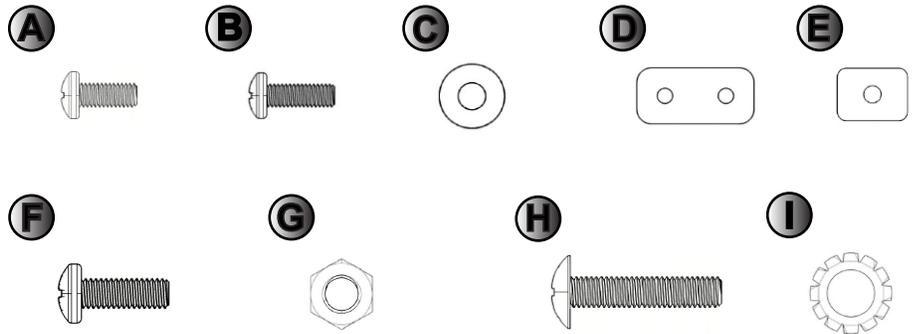
Step 1. Assemble (1) M4X10mm screw, (1) M4 washer and (1) Rectangle T-slot nut through the bottom hole of the Bent Acrylic as shown below:
