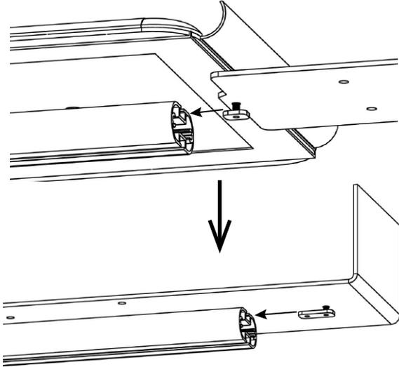
Step 4. Assemble (1) M4X10mm screw, (1) M4 washer and (1) Rectangle T-slot nut at the lower hole of the Top Acrylic. Remove the end cap from the top of the pole. Pivot the snap frame to the side.
