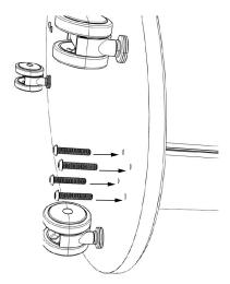
Tips: Do not tighten one screw at a time. Thread in all 4 screws first, then tighten all the screws together.
