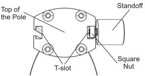
4. Place the top standoff 4" down from the top of the pole, then tighten the standoff to the pole by using the provided hex wrench. Fix the top standoff on the other side. Make sure both top standoffs are on the same level.
