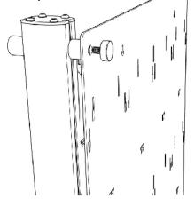
Screw in the caps tightly to all of the standoffs to fix the board completely.
