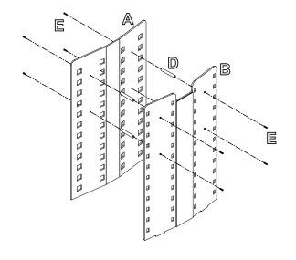
Step 1. Connect the Front Panel (B) and the Back Panel (A) Step 2. Connect the the assembled display body with Base (C) by inserting the tabs on the front panel into the cutouts on the base. Secure the back panel onto the base by using 4 M4 screws (E).
