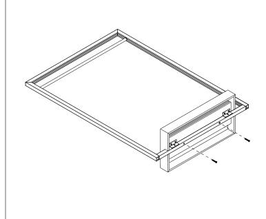
STEP 2. Use M8x50 Screws (C), M8 Nuts (D) and Washers (H) to secure the base with the metal frame as shown. Tighten the screws and nuts with Allen Wrench (G) and M8 Wrench (I). Connect the power adapter with the power cable on the metal frame.
