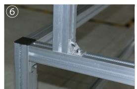
Slowly lay the assembled frame onto the ground on its side. Insert nuts into T-slots at the bottom and then attach the Casters (G) by threading the post of the casters into the bottom of the frame. See Image 10. Secure all 6 casters at the bottom close to the side frames.
