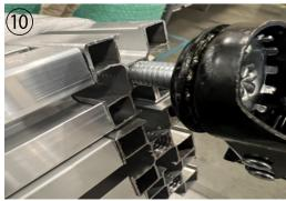
Assemble 1 Corner Bracket (E) by sliding the nut into T-slot of the Framing Rail (C). Make sure the side of the bracket is flush with the end of the framing rail, then tighten the screw to fix the bracket at the position. Repeat the step to attach 1 corner bracket at each end on all Framing Rail C.
