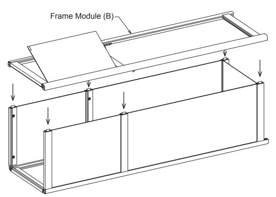
Secure the Frame by tightening all screws in the aluminum bars that connecting with Frame Module with Door (B).
