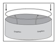
With the help of another person rest the 2nd ring on top of the middle supports and drape the banner over the ring. Make sure to keep the banner, ring, and support holes aligned.
