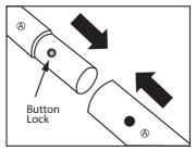
Connect (5) Long Bars (A) end to end to form a closed ring. Repeat this step to form another ring. These are the top and bottom supports for your graphic.
