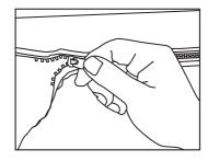
Once all long screws are in place, lift the inside of the graphic and zipper The sections together.
