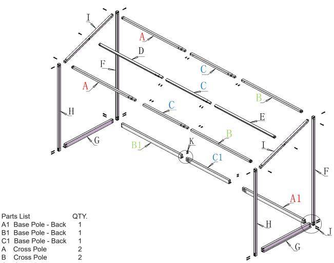
Cross Pole 3 С D Cross Pole 1 Ε Cross Pole 2 F Leg Post - Back 2 G Base Pole - Side Leg Post - Front 2 2 Т Rafter Pole M6x35 screw 22 J K M6x16 screw 16 Allen key 1 M Fabric Canopy 1 Edge Clamp 5
