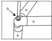
Using the short screws (D) attach the Short Bar (B) to each corner as pictured.
