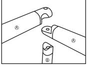
Align the ends of the each side as show, making sure to align the groves in each piece to properly align.
