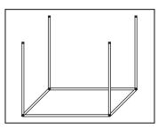
Set the assembled base on the ground so that the Short Bars are facing upward.
