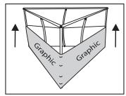
With the help of another person, position your graphic so the center seam is centered with the bottom frame and the corners are aligned. Raise the graphic up and over the outside of the frame.
