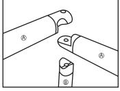
Align the ends of the each side as show, making sure the groves in each piece properly align.
