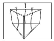
Attach the 2nd set of long bars (A) to the top of the curved short bars (E) using the remaining short screws (D). Align the corners but do not attach.
