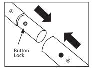
Connect (1) A-Left and (1)A-Right together to make a side of your triangle. Do this 6 times to construct the sides of your triangle.
