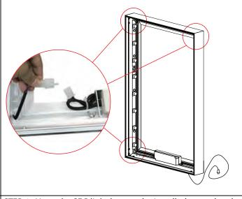
STEP 4. Hang the SEG light box on the installed upper brackets. Tighten the wing nuts on the upper brackets first. Install the lower brackets and tighten the wing nuts on the lower brackets.
