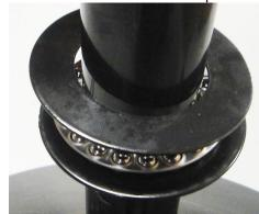
Drop (1) collar onto the bearing assembly through the pole as shown below.
