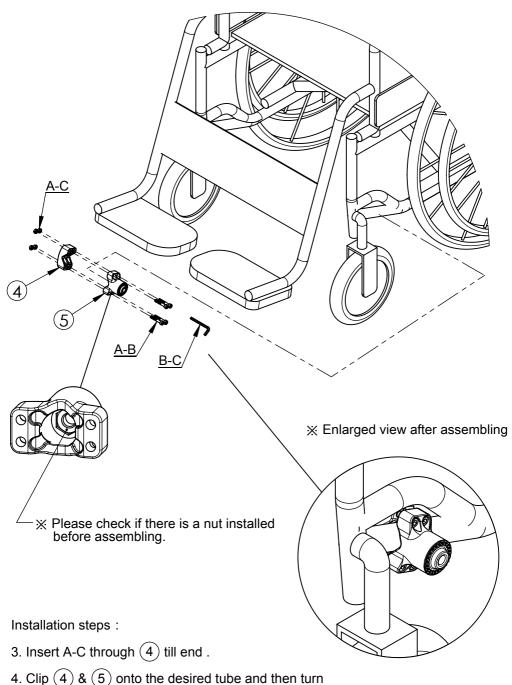
4. Clip 4 & 5 onto the desired tube and then turn A-B until tight.
