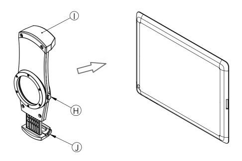
Attachment Description 1 : Press H and stretch J till larger than the length of tablet. Then release H .
