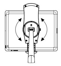
Attachment Description 5 : After attaching, turn tablet clockwise or anti-clockwise to get the best view.
