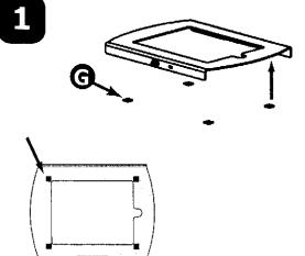
Attach four small 1.5mm thick foam pads to underside of cover as shown above.
