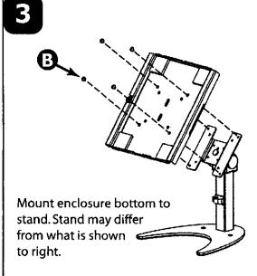
If mounting to IPAD135 use four M5 socket head screws (B) attaching bottom of iPad enclosure to stand with Hex key (C).
