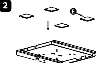
Attach four 3mm foam pads in enclosure bottom.
