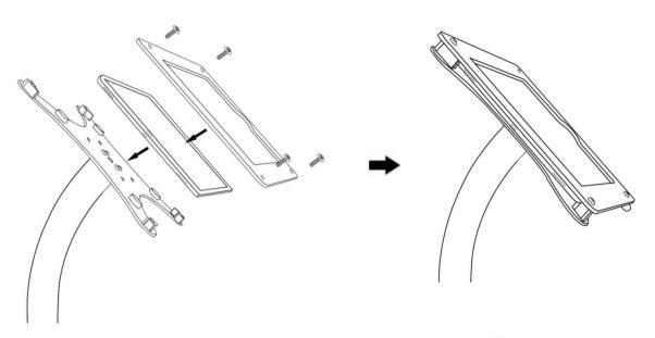
When put the tablet, the **Earphone jack** should be on **C corner** if you want to attach earphone or card reader.
