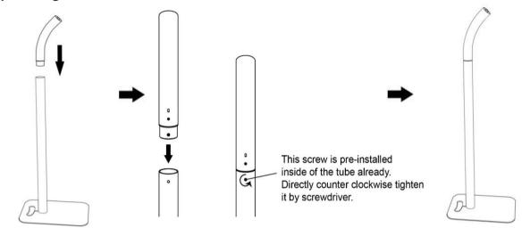
Insert the bended tube Remember Counter clockwise tightening Ready for next step feed the cable to the bended tube the screws of both sides using **Hex end screwdriver**
