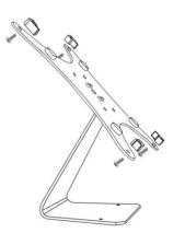
Do not fully tighten all screws! Need to adjust in next step. Step3Add your Tablet PC and add the Acrylic cover using 4pcs Screw "a".Fully tighten all screws after installed all parts correctly.
