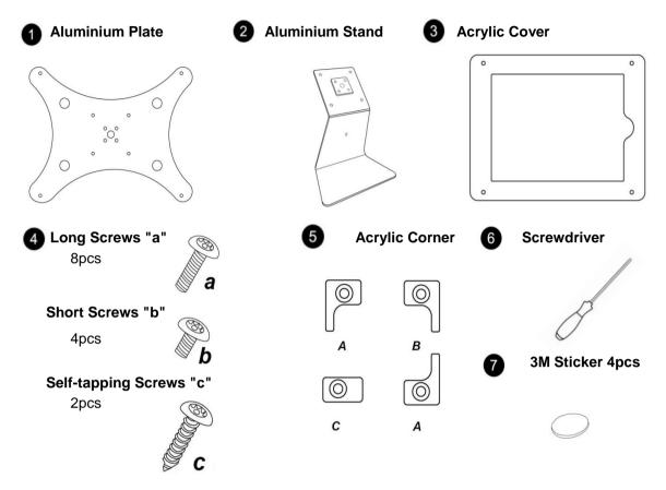
**Step1** Connect the **Aluminium Plate** to the **Aluminium stand** using 4pcs **Screw "b"**
