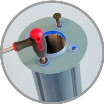
Loosely Insert 2 screws through aligned diametrically opposite holes. Fully tighten 1 screw using hex key provided before removing second screw.
