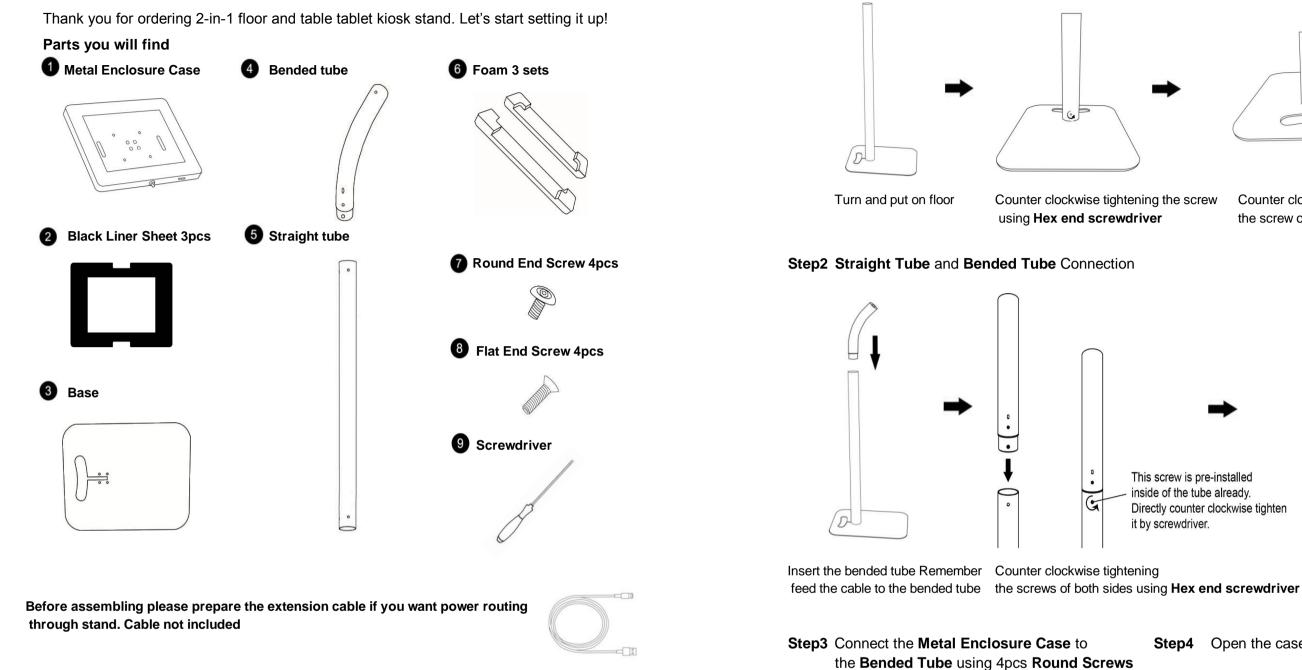
Step1 Base and Straight Tube Connection Please remember to insert cable when install if need power routing.
