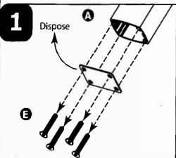
Remove the screws (E) from the bottom of the post (A). Save the screws (E) for step 2. Dispose of the small steel plate.
