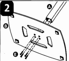
Attach the base to the bottom of the post assembly (A) using the removed flat head screws (E) and allen wrench (F).
