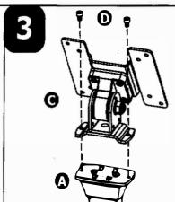
Attach the rotating bracket (C) to the top of the post assembly using the supplied socket head screws (D) and allen wrench (F).
