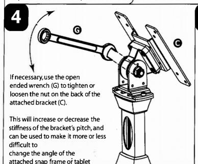
The holes in the bracket at the top of the stand are threaded to accept M5 screws. Use these holes to mount tablet holders or other accessories to the stand using the appropriate hardware included with those kits.
