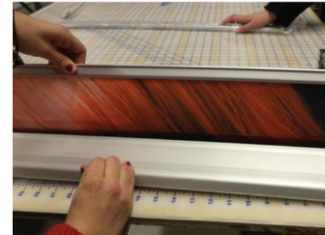
**6.** Pull the Allen Key while holding on to the attached graphic. Save the Key in the base side cover, which is magnetic and will secure the Key. Put the side cover back on.
