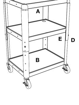
Position the bottom shelf **B** so that the caster holes are facing up. Insert caster **C** into the caster holes on the bottom of shelf **B**. Use a mallet to set the casters properly.
