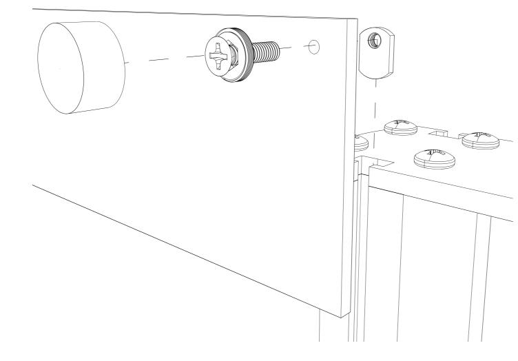
2. If mounting to a wall use the panel as a template for the hole locations. Drill and insert the wall anchor. Thread the screw through the brass fitting, through the panel into the wall anchor. Screw stainless steel caps onto brass fitting.
