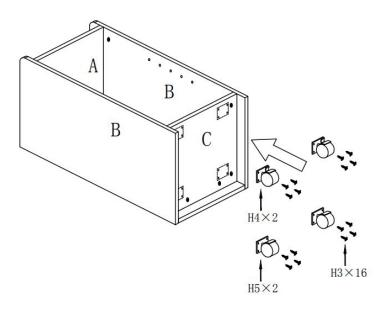
4. Line up casters with the guide holes on the bottom of panel C. Then, tighten screws to secure casters to the unit.
