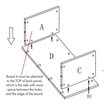
Insert cam posts into back panel, then fit top and bottom panel onto posts. Then, insert cam locks and tighten to secure.
