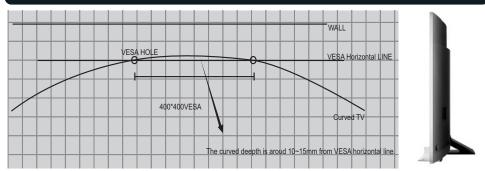
NOTE:To install curved TV,please use "M8\*30 screw+big spacer(15mm) or big&small(20mm) Spacer together" NOTE:To install curved TV,please use "M8\*50 screw+big&big spacer(30mm) or big&big&small spacer(35mm) or big&big&small(40mm) Spacer together"
