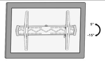
Push or pull from the top or bottom of the screen to obtain the desired angle.
