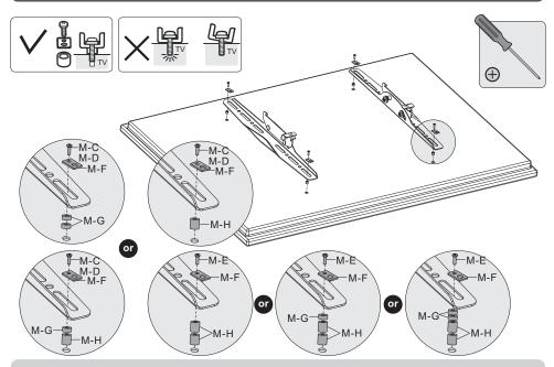
Note: Choose appropriate screws, washers and spacers (if necessary) according to the type of screen.
