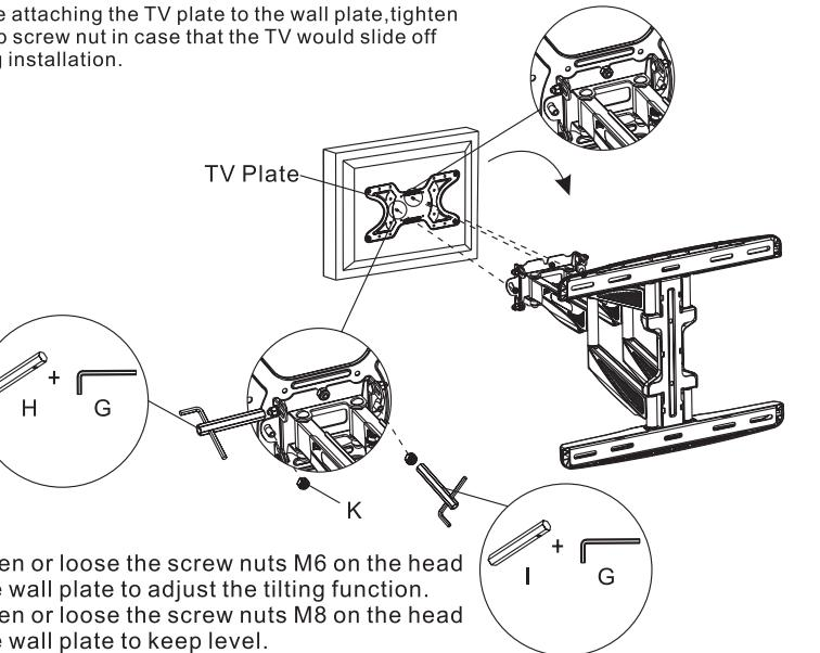
Tighten or loose the screw nuts M6 on the head of the wall plate to adjust the tilting function.
