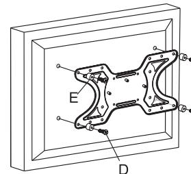
Attaching TV plate to screen with recessed back
