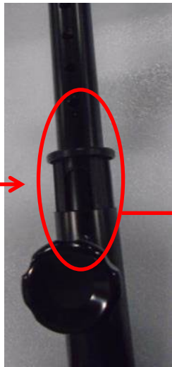
STEP 3 Extending the Pole (1). Plus the Long knob Screw.
