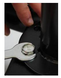
Place in all (4) bolts with "48" label on top, and screw in with one of the provided wrenches.
