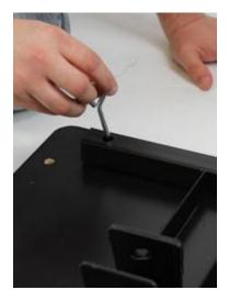
Screw in short bolts to secure shelf mount bracket.
