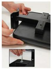
Place the second shelf top face down, and line up bracket mount with predrilled holes. Place washers on top of the holes, and then use long screws to put it in place.
