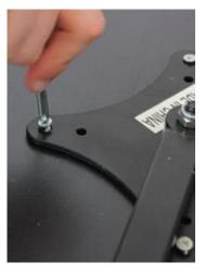
Place shelf top face down, and line up bracket mount with predrilled holes, and then use short screws to put it in place.
