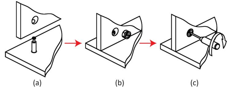
1. Place the top wood panel on the soft surface with pre-drilled holes facing up. Screw in 4 cam posts (A) with phillips screw driver, and insert 2 dowels (B) as shown below.
