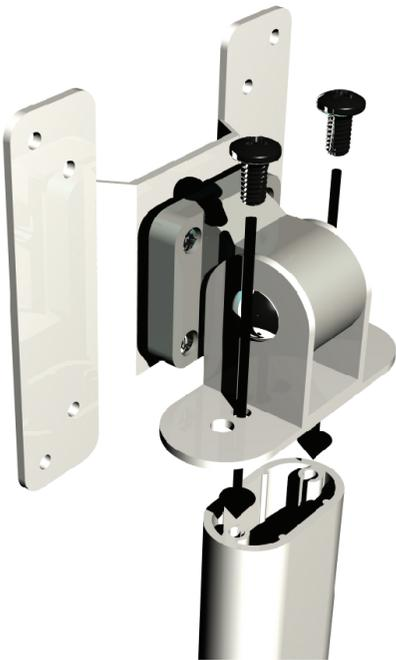
Insert screws B through adapter bracket and into pole.
