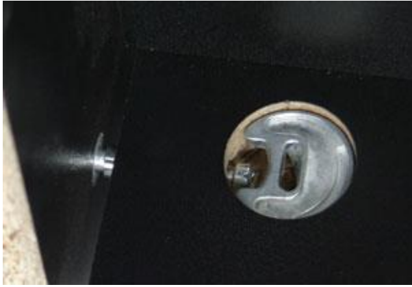
Proper alignment of cam lock. Using a flathead screwdriver, turn clockwise to tighten
