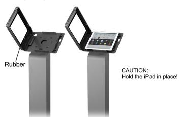
4. Connect the charging cable with the iPad. Then close the cover and securely lock it to the enclosure.
