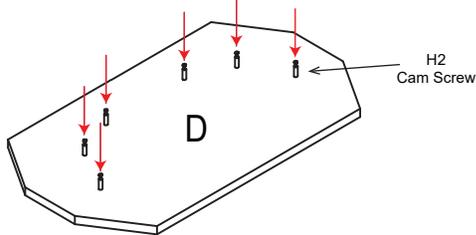
Attach assembled podium body to base panel (D) by inserting cam posts into the cam lock holes.
