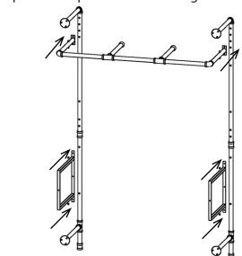
**Step 3.** Attach the assembled rack to the wall. Mark drill locations through holes on mounting plates. Drill holes, then fix the rack with stud anchors. (See Page 2 for drill size)
