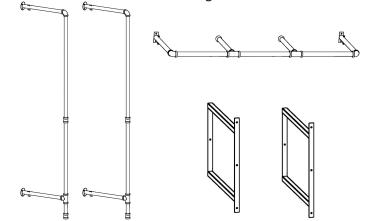
**Step 2.** Fix spoked hanging bar and shelf brackets on to two poles with provided screws. Tighten all screws.
