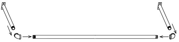
**Step 2.** Attach the assembled Hanging Bar in Step 1 to (2) Wall Mount Pole (PPLNOUTRIG) at desired height. Align holes on rectangle plates with holes on Wall Mount Pole. Screw in all provided screws (Part E) on both sides with Hex Key (Part F)
