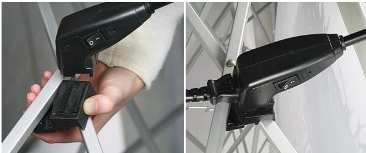
After your graphics are installed you can add the optional floodlights. Lights can only be installed at the intersection of two horizontal frame poles. Make sure the channels on the bottom of the clip are seated on the poles and are firmly snapped into place. After the clip is attached to the frame, slide the light onto the channels in the clip. See picture above left.
