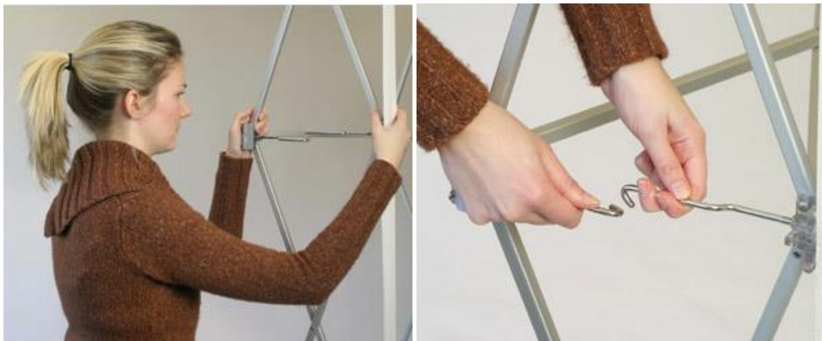
Connect all of the hooks in the frame as shown above. This will keep your frame from collapsing. If you find it easier, you can also lay the frame on the ground to do this step.
