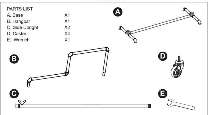
Step 1. Screw (4) Casters into the base using the wrench provided with the unit. Tighten all Casters to secure the cloth rack.
