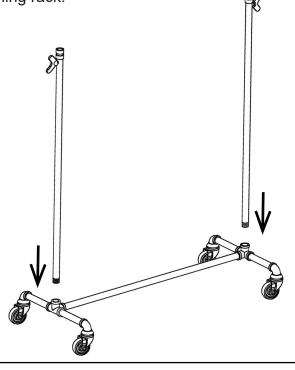
Step 3. Keep the assembly upright. Twist wing nuts on uprights to loosen adjustable connectors. Align Top Hangbar with side uprights as shown, then Insert hangbar into uprights. Drop and lock
