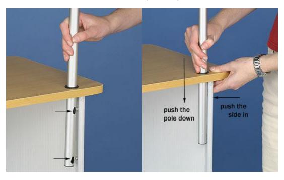
Insert each pole into the two holes in the countertop. Be sure that the Velcro® patches on the poles face front to hold the header. Line up the holes in the poles with the screws in the plastic frame. See picture left. Insert the screws into the holes, and then push down on the poles to latch them firmly in place. You may also need to push in on the plastic sides to make sure these pieces are properly connected.
