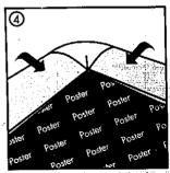
After placing the cover back on the poster, close the profiles downwards.
