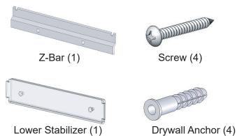
1. Place z-bar in desired location on a wall and mark the holes using a pencil. Remove z-bar and drill two 7/32" holes. Insert anchors and attach z-bar with screws.
