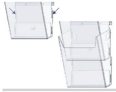
b). To get full view display, attach inserts into the lower slots. Repeat for remaining pockets.
