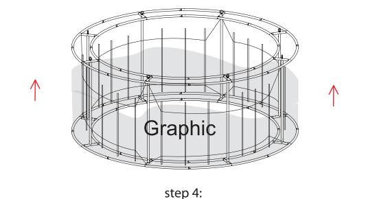
Place the graphic cover at the bottom of the frame.
