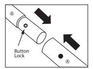
Connect (7) Long Bars (A) end to end to form a closed ring. Repeat this step to form another ring. These are the top and bottom supports for your graphic.
