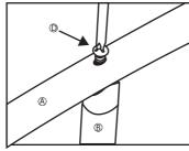
Attach ring to middle supports (B) using the short screws (D).
