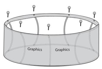
Align all holes then insert long screw and hand tighten.
