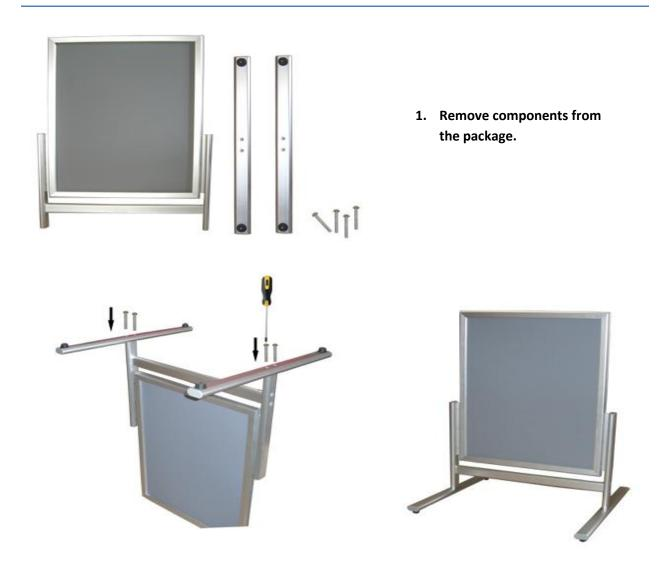
2. Screw the two feet to the snap frame with a screwdriver.
