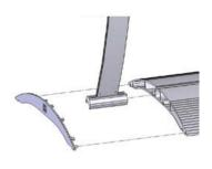
**4.** Slide the second side support into the base and secure it in place with a screwdriver. (Please remember to connect the poster bar as well.) Replace end cap.
