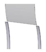
**5.** Insert poster and lenses (at the same time) into the grooved channels. Make sure the bottom portion of the poster slides into the bottom bar.
