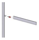
**3.** Measure and attach lower poster connectors to both extrusions. Slide the bar onto the connector.
