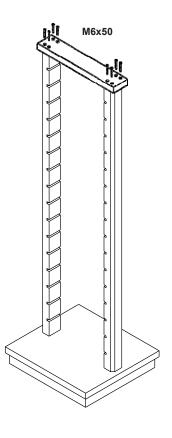
Fix the partition /top rail to the poles on top with screws.
