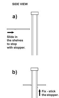
Beware of stoppers in position as shown (from below). After positioning the shelves, fix it with stopper on other side.
