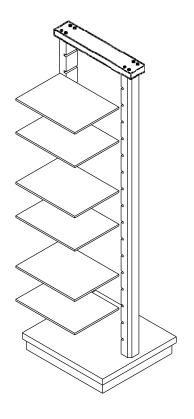
Slide the glass shelves into channels (choose requested position). Stoppers prepared to stop the slide on one side.
