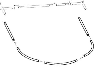
2. Hold the assembled tube with mounting brackets at the desired mounting location on the wall. Mark the center through the hole with a pencil. Keep the tube level using a bubble level.
